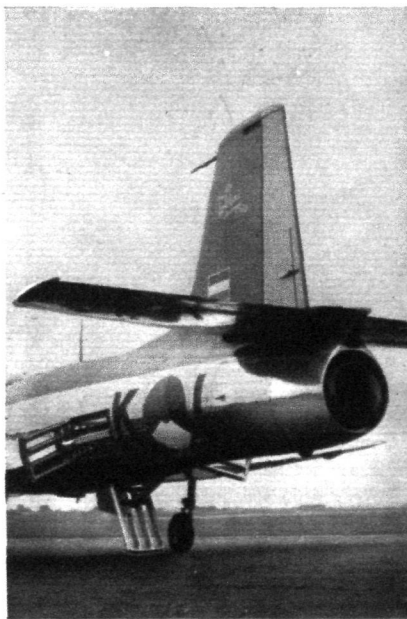
On the left is the tail of the S.14 Nene with larger jet-pipe, modified lines, and new three-section lattice-type air brakes extended. For comparison the earlier S.14 Derwent tail is illustrated on the right.
